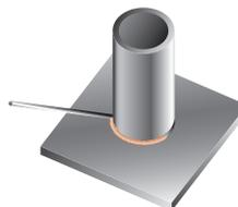
PB TUBE FIXE. L'AXE DU TUBE EST VERTICAL.
