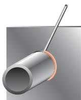
PF TUBE FIXE. L'AXE DU TUBE EST HORIZONTAL.
